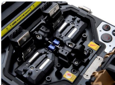
Precise structural design Core to core alignment
